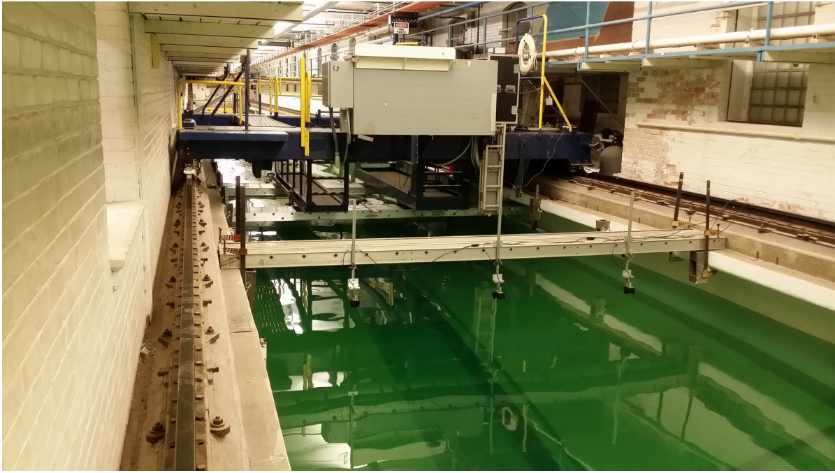
Figure 6: Carriage in WEC testing configuration and upstream wave probes
